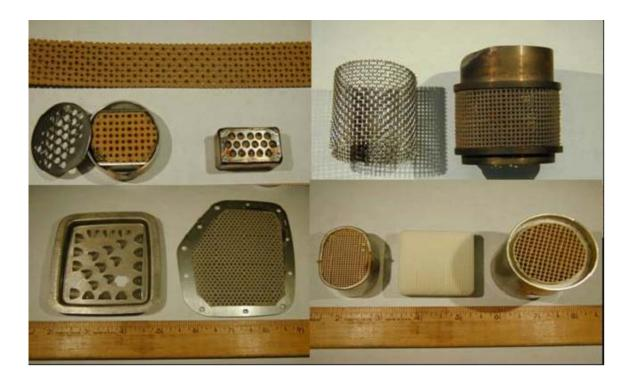
**Figure 4.** Small engine catalysts and substrates can take on many shapes and sizes, from perforated plates and coated screens to mini honeycombs.
