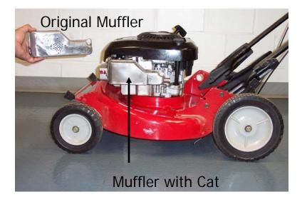
Figure 5. Catalyst engineered and integrated to fit inside existing muffler of Class I engine.<sup>8</sup>
