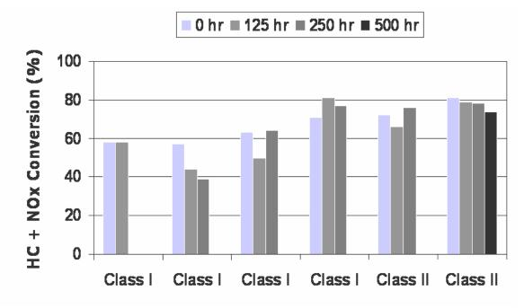
Figure 8. Catalyst HC+NOx Efficiency versus Operating Hours<sup>8</sup>
