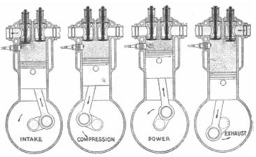
**Figure 1.** Four-Stroke Combustion Cycle<sup>6</sup>
