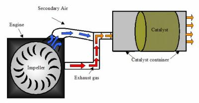
Figure 7. Venturi Passive Secondary Air System<sup>8</sup>
