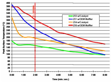
Figure 11. Hot soak peak surface temperatures on Class II tractor following 30 min. of operation.<sup>9</sup>
