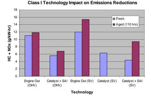
Figure 9. Emissions from Class I engine employing different control technologies.
